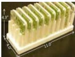
Petri plate holder with Arabidopsis petri plates inserted.
