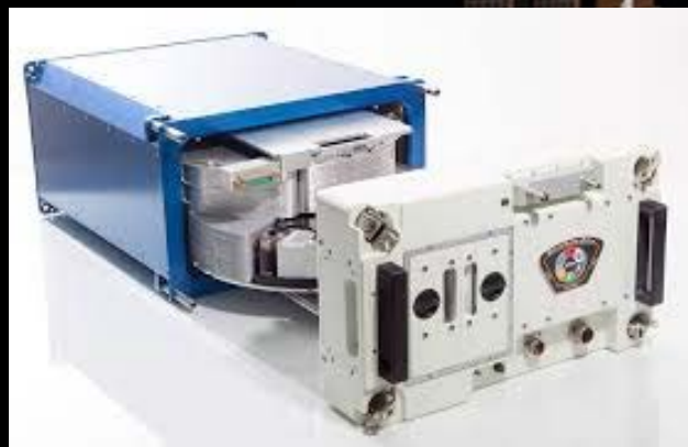
Techshot Multi-Use Variable-g Platform (centrifuge systems for Plants, invertebrates, Cells, Microbes)
