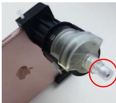
The device is portable and can 1) connect to a mobile phone to perform blood analysis and 2) store data
