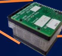
Biosensor payload with fluidic cards and optical sensors
