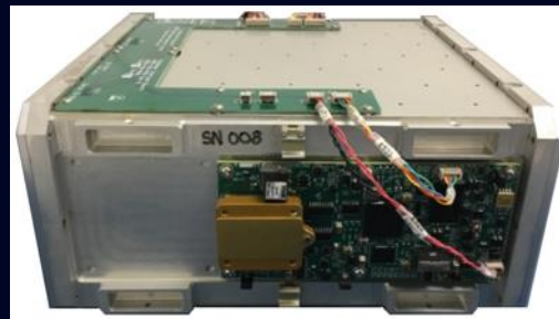
LET spectrometer attached at one end of payload
