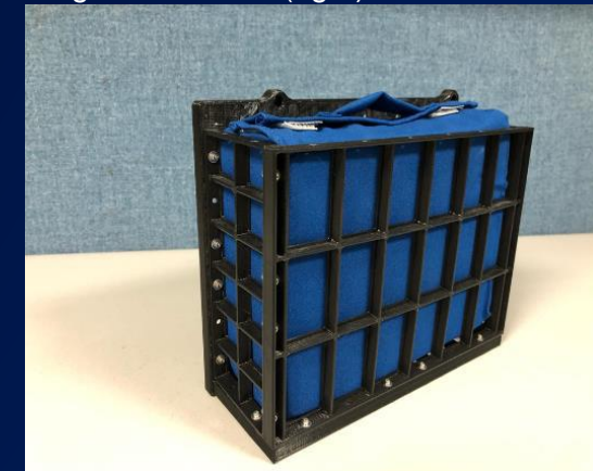
3D printed 1/2 scale mockup of SBP Payload Container Assembly with blue Science Bag contained within.
