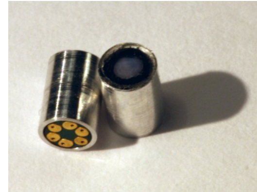
IOC with lens and image sensor awaiting haptic elements
